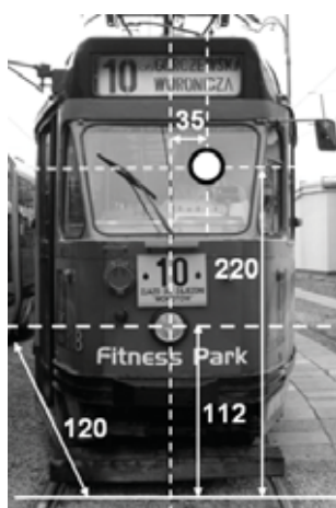
Fig. 1. Tram 13N with a single reflector 0215.8.10.8.0 produced by Zelmot (with a H4 light bulb)
