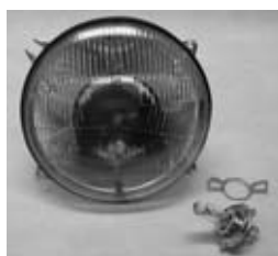
Fig. 4. Lamp 0215.8.10.8.0 produced by Zelmot with a H4 light bulb installed on tram 13N
