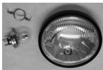
Fig. 5. Lamp 0245.2008.1 produced by Zelmot with a R2 light bulb installed on tram 105N
