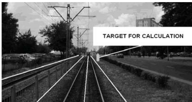
Fig. 13. Position of the target on the tram's foreground (the lines indicate the limiting outline of tramline and the axis of tram's trajectory)
