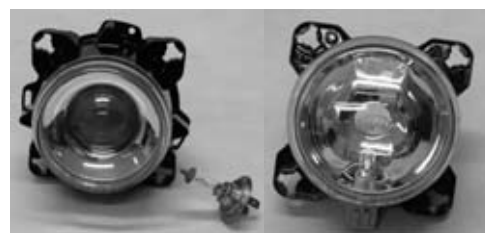
Fig. 6. Low beam light projector (left) 1BL 008 193-01 and reflector FF of main lights (right) 1KO 008 191-02 produced by Hella with H7 light bulbs installed on tram 120N
